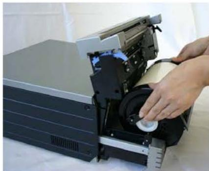
9. Turn the paper in the direction of the arrow. When it is advanced enough, the buzzer will beep, and the flashing LED (orange) will go out.
